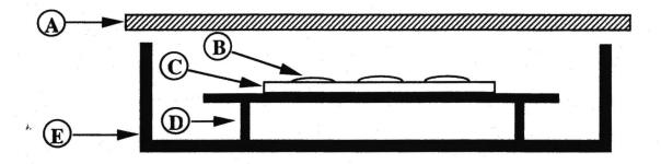
box was equipped with a window (28 cm X 21 cm). Samples were affixed to a cardboard platform raised to 0.5 cm below window level (Fig. 2). When the samples were exposed to full spectrum sunlight, a single layer of Saran Wrap, which transmits all solar UV wavelengths (Fig. 1), was placed over the window. To filter out the UV-B portion of sunlight, the window was covered with 1/2 inch thick plate glass, which was opaque to UV wavelengths of 320 nm or shorter (Fig. 1).
