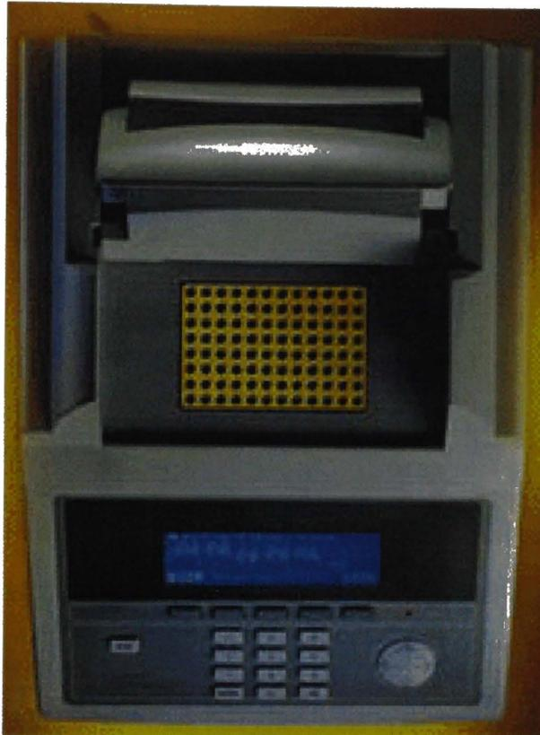
Figure 1 – The GeneAmp® PCR System 9700 thermal cycler. Picture shows the gold-plated silver block in place. Courtesy Applied Biosystems, Foster City, CA. <http://www.appliedbiosystems.com>
