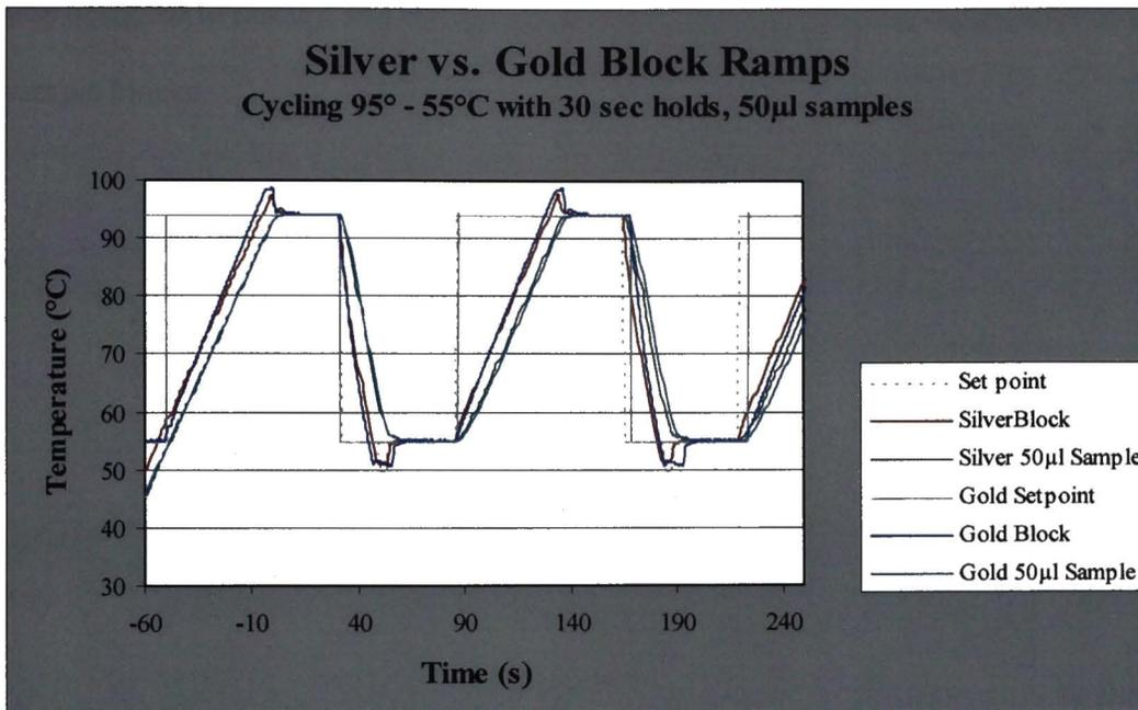
**Figure 3** – A comparison of the silver and gold-plated silver block ramping profiles. Courtesy Applied Biosystems, Foster City, CA.
