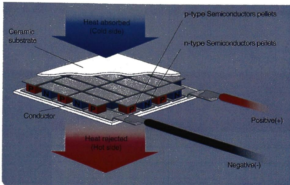
**Figure 2** – Peltier thermoelectric module. <http://www.inbthermoelectric.com>
